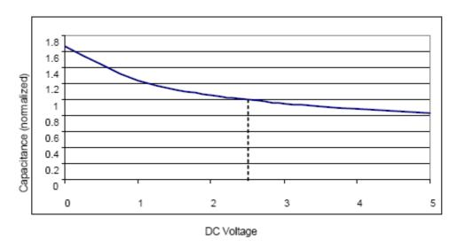
Figure 5. Filter Capacitance vs. Input Voltage (normalized to capacitance at 2.5 VDC and 25°C)
