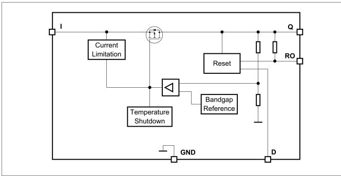
Figure 2 Block Diagram TLS810C1
