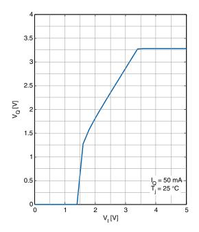
Load Regulation  $\Delta V_{\mathbf{Q}, \mathrm{line}}$  versus Input Voltage  $V_{\mathbf{I}}$
