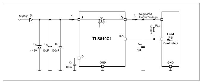
Figure 7 Application Diagram
