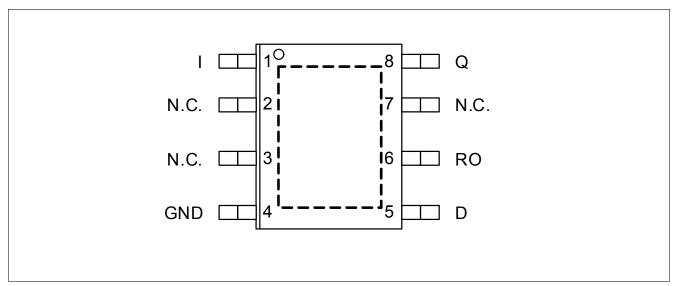
Figure 3 Pin Configuration TLS810C1 in PG-DSO-8 EP package
