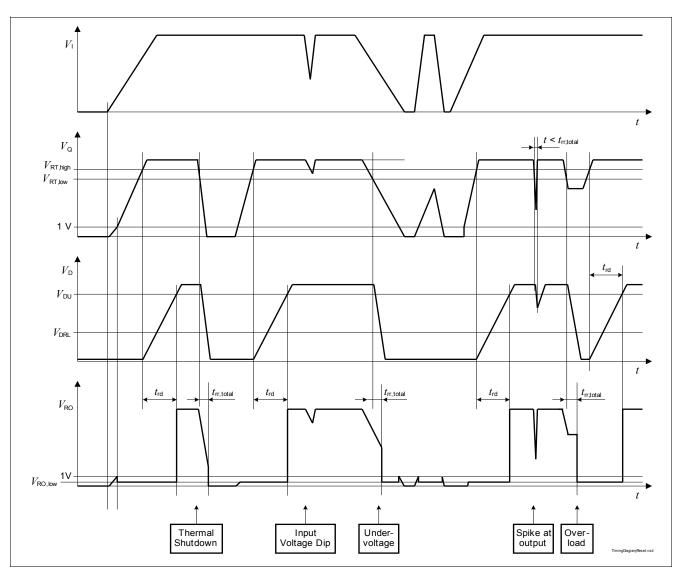
Figure 6 Timing Diagram Reset
