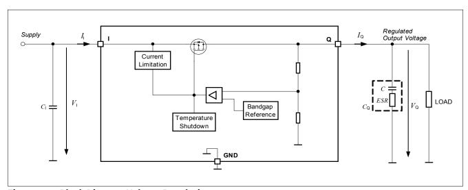
Figure 4 Block Diagram Voltage Regulation
