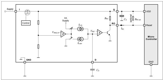
Figure 5 Block Diagram Reset Function
