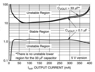
Figure 8. Output Stability with Output Capacitor Change
