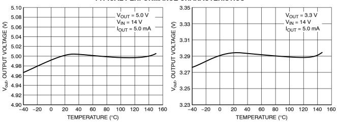
Figure 3. 5 V Output Voltage vs Temperature
