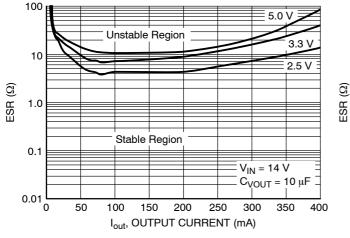
Figure 7. Output Stability with Output Voltage Change
