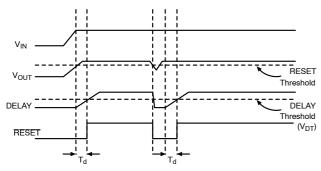
Figure 13. Reset and Delay Circuit Wave Forms
