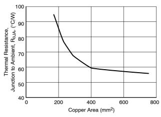
Figure 20. 16 Lead SOW (Exposed Pad),  $\theta$ JA as a Function of the Pad Copper Area (2 oz. Cu Thickness), Board Material = 0.0625" G-10/R-4
