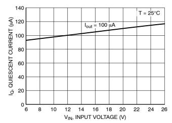
Figure 11. Quiescent Current vs Input Voltage
