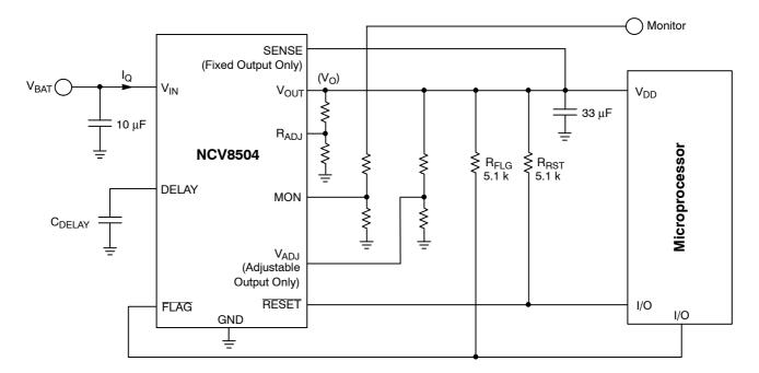
Figure 1. Application Diagram
