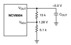
Figure 16. Adjustable Output Voltage
