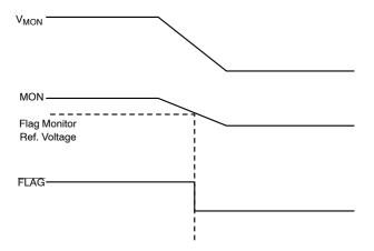
Figure 17. FLAG Monitor Circuit Waveform
