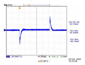
Figure 14. Vin=12V, Vout=5V, BW~50kHz
