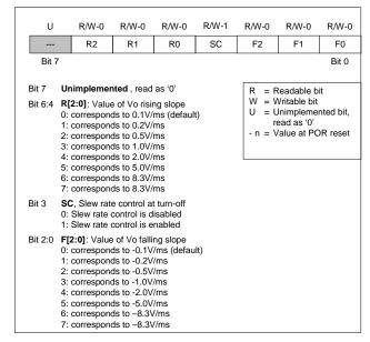
Figure 34. Tracking Configuration Register TC
