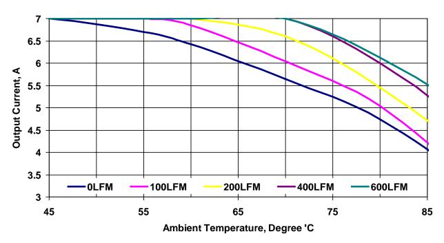
Figure 21. Thermal Derating Curves. Vin=12V, Vout=5.0V, Fsw=1MHz
