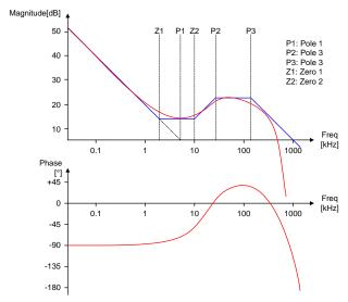
Figure 52. Transfer Function of PWM
