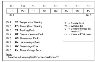
Figure 35. Protection Status Register ST
