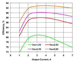
Figure 4. Efficiency vs. Load. Vin=9.6V, Fsw=500kHz
