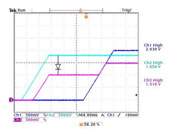
Figure 11. Turn On into Prebiased Load. V3 is Prebiased by V2 via a Diode.
