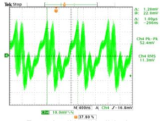
Figure 47. Input Voltage Noise, No Interleave
