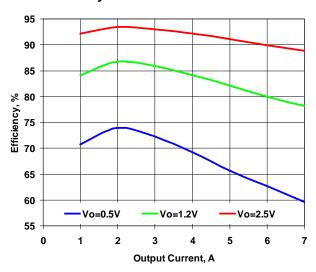
Figure 2. Efficiency vs. Load. Vin=3.3V, Fsw=500kHz
