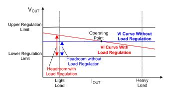
Figure 27. Optimal Voltage Positioning Concept
