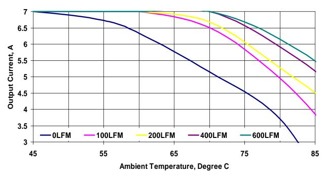
Figure 20. Thermal Derating Curves. Vin=14V, Vout=5.0V, Fsw=500kHz
