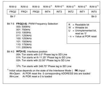
Figure 46. Interleave Configuration Register INT
