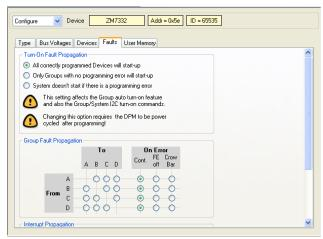
Figure 42. DPM Configure Faults Window
