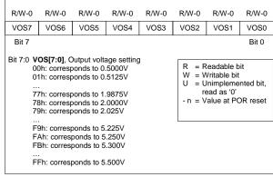
Figure 26. Output Voltage Setpoint Register VOS
