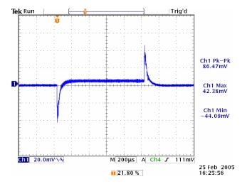
Figure 17. Vin=5V, Vout=1V, BW~40kHz
