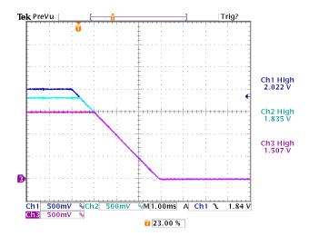
Figure 12. Tracking Turn-Off. Falling Slew Rate is Programmed at 0.5V/ms.
