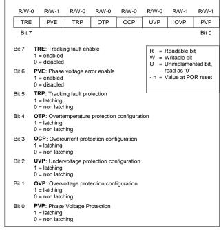
Figure 39. Protection Configuration Register PC1
