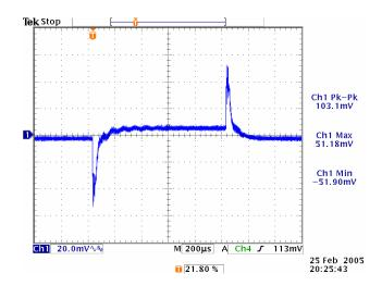
Figure 16. Vin=5V, Vout=2.5V, BW~40kHz
