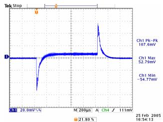
Figure 18. Vin=3.3V, Vout=1V, BW~40kHz
