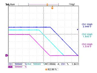
Figure 13. Turn-Off with Tracking and Sequencing. Falling Slew Rate is Programmed at 0.5V/ms.
