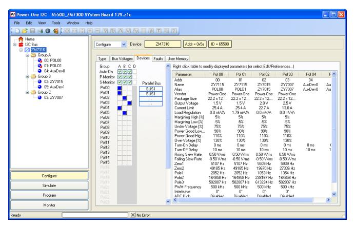
Figure 53 DPM Configure Devices Window
