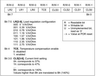
Figure 36. Current Limit Setpoint Register CLS
