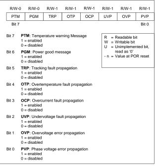
Figure 41. Protection Configuration Register PC3
