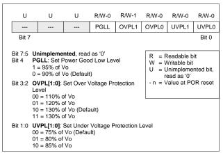
Figure 37. Protection Configuration Register PC2
