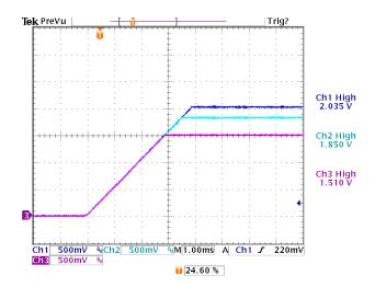
Figure 8. Tracking Turn-On. Rising Slew Rate is Programmed at 0.5V/ms.
