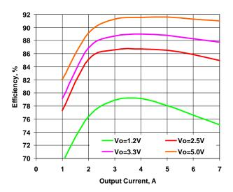
Figure 5. Efficiency vs. Load. Vin=12V, Fsw=500kHz
