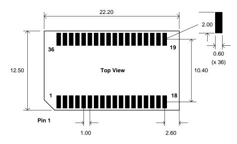
Figure 58. Recommended PCB Pad Sizes
