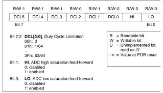
Figure 51. Duty Cycle Limit Register
