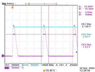
Figure 44. Turn-On into UVP on V3. The UV Fault Is
