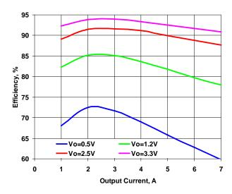
Figure 3. Efficiency vs. Load. Vin=5V, Fsw=500kHz
