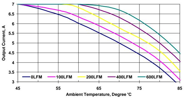
Figure 22. Thermal Derating Curves. Vin=14V, Vout=5.0V, Fsw=1MHz
