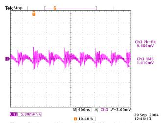
Figure 50. Output Voltage Noise, Full Load, 180° Interleave
