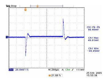
Figure 15. Vin=12V, Vout=1V, BW~40kHz
