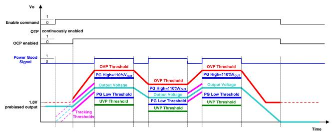
Figure 40. Protection Enable Conditions
