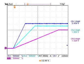
Figure 9. Turn-On with Different Rising Slew Rates.
