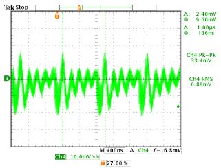
Figure 48. Input Voltage Noise with Interleave
