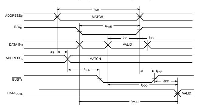
Figure 12. Write Timing with Busy Input (M/S=LOW)
