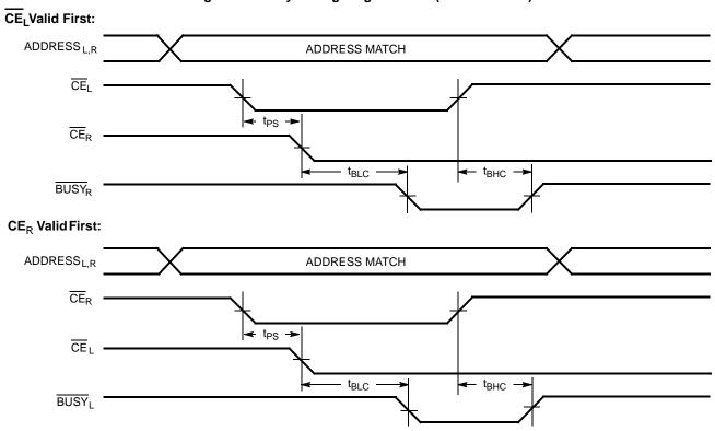
Figure 14. Busy Timing Diagram No. 2 (Address Arbitration)<sup>[34]</sup>
