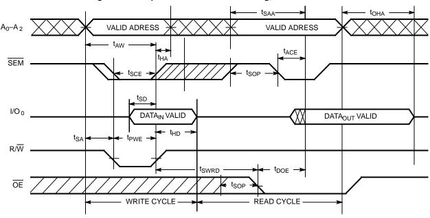
Figure 10. Timing Diagram of Semaphore Contention  $^{[30,\ 31,\ 32]}$
