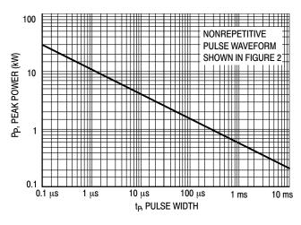
Figure 1. Pulse Rating Curve
