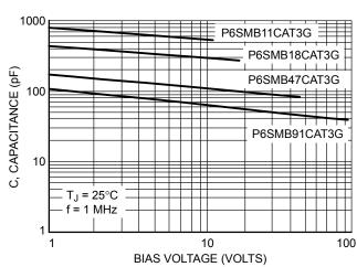
Figure 4. Typical Junction Capacitance vs. Bias Voltage
