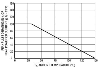
Figure 3. Pulse Derating Curve
