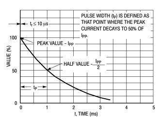
Figure 2. Pulse Waveform
