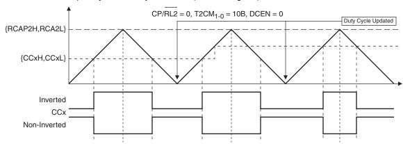
Figure 13-11. Phase Correct Symmetrical (Center-Aligned) PWM
