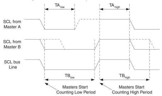
Figure 18-7. SCL Synchronization between Multiple Masters
