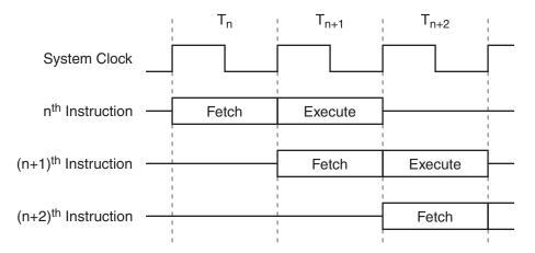
**Figure 5-2.** Single-cycle ALU Operation (Example: INC R0)
