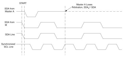
Figure 18-8. Arbitration between Two Masters
