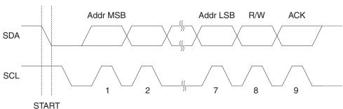
Figure 18-4. Address Packet Format
