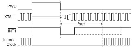
When PWDEX = "1", the wake-up period is controlled externally by the interrupt. Again, at the falling edge on the interrupt pin, power-down is exited and the oscillator is restarted. However, the internal clock will not propagate until the rising edge of the interrupt pin as shown in Figure 8-2. The interrupt pin should be held low long enough for the selected clock source to stabilize. After the rising edge on the pin the interrupt service routine will be executed.
