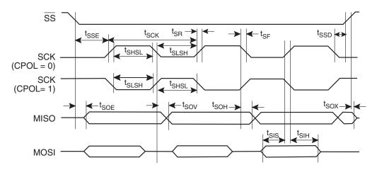
Figure 26-19. SPI Master Timing (CPHA = 1)
