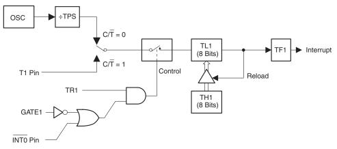
Note: RH1/RL1 are not required by Timer 1 during Mode 2 and may be used as temporary storage registers.
