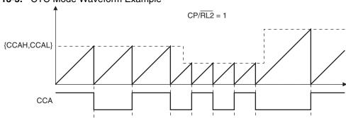
Figure 13-5. CTC Mode Waveform Example
