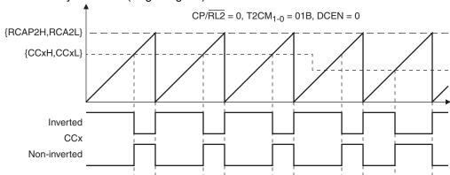
Figure 13-8. Asymmetrical (Edge-Aligned) PWM
