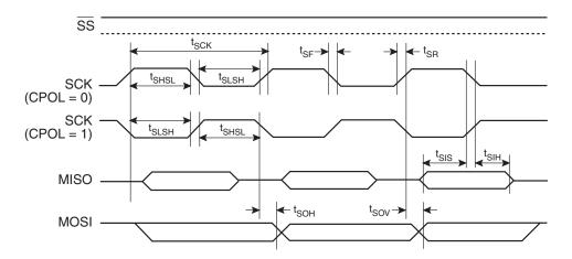
Figure 26-20. SPI Slave Timing (CPHA = 1)
