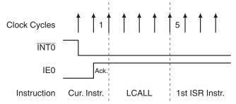
Figure 9-2. Maximum Interrupt Response Time
