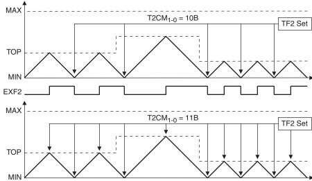
Figure 12-7. Timer 2 Waveform: Dual Slope Modes
