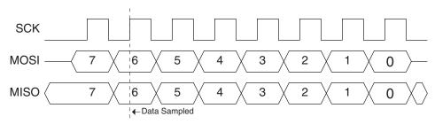
Figure 25-12. Serial Programming Interface Timing
