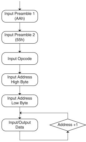
Figure 25-5. ISP Command Packet (Serial)
