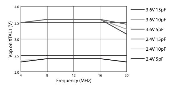
Note: 1. Replacing capacitor C1 with a resistor R1 of 4  $M\Omega$  results in similar swing levels on XTAL1.
