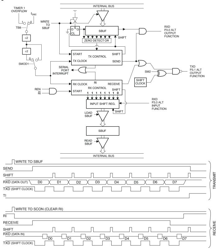
Figure 16-2. Mode 0 Waveforms
