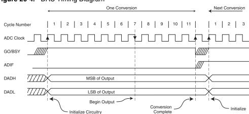
Figure 20-4. DAC Timing Diagram
