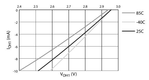
Figure 26-10. Push-Pull Output I-V Sink Characteristic at 3V
