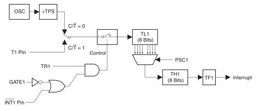
Mode 0 operation is the same for Timer 0 as for Timer 1, except that TR0, TF0, GATE0 and INTO replace the corresponding Timer 1 signals in Figure 11-1. There are two different C/T bits, one for Timer 1 (TMOD.6) and one for Timer 0 (TMOD.2).
