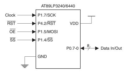
The Programming Interface is the only means of externally programming the AT89LP3240/6440 microcontroller. The Interface can be used to program the device both in-system and in a standalone serial programmer. The Interface does not require any clock other than SCK and is not limited by the system clock frequency. During Programming the system clock source of the target device can operate normally.
