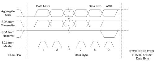
Figure 18-5. Data Packet Format
