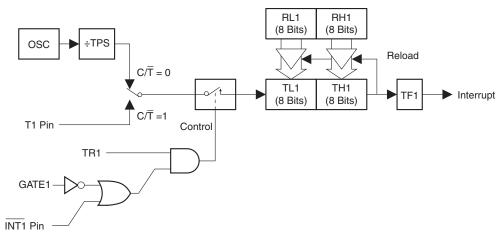
Figure 11-2. Timer/Counter 1 Mode 1: 16-bit Auto-Reload
