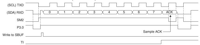
Mode 0 transfers data LSB first whereas SPI or TWI are generally MSB first. Emulation of these interfaces may require bit reversal of the transferred data bytes. The following code example reverses the bits in the accumulator:
