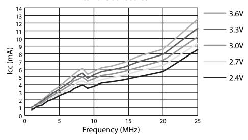
Figure 26-6. Idle Supply Current vs. Frequency
