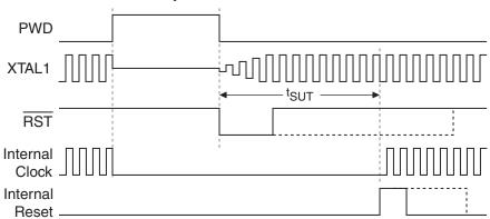
Figure 8-3. Reset Recovery from Power-down
