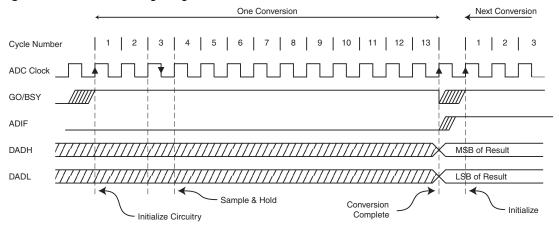
Figure 20-2. ADC Timing Diagram
