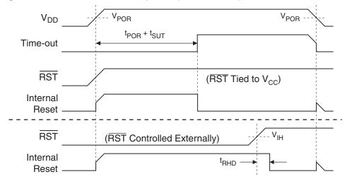
If the Brown-out Detector (BOD) is also enabled, the start-up timer does not begin counting until after  $V_{DD}$  reaches the BOD threshold voltage  $V_{BOD}$  as shown in Figure 7-2. However, if this event occurs prior to the end of the initialization sequence, the timer must first wait for that sequence to complete before counting.
