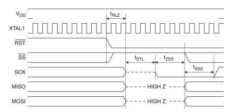
Figure 25-9. In-System Programming (ISP) Start Sequence
