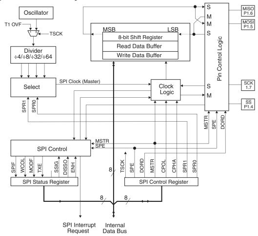
Figure 17-1. SPI Block Diagram
