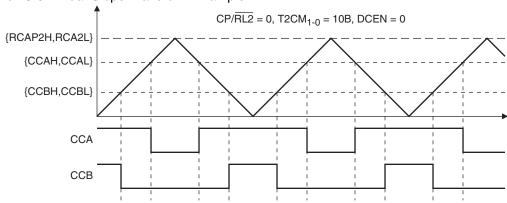
Figure 13-6. Dual-Slope Waveform Example
