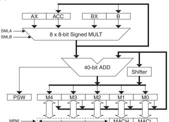
The MAC operation is performed by executing the MAC AB (A5 A4H) extended instruction. This two-byte instruction requires nine clock cycles to complete. The operand registers are not modified by the instruction and the result is stored in the 40-bit M register. MAC AB also updates the C and OV flags in PSW. C represents the sign of the MAC result and OV is the two's complement overflow. Note that MAC AB will not clear OV if it was previously set to one.
