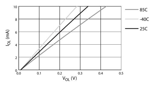
Note: The  $I_{OL}/V_{OL}$  characteristic applies to Push-Pull, Quasi-Bidirectional and Open-Drain modes.
