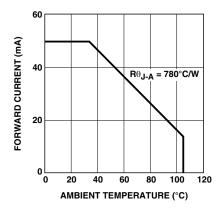
Figure 5. Maximum forward DC current vs. ambient temperature.
