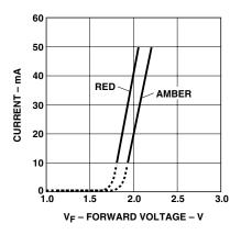
Figure 3. Forward current vs. forward voltage.
