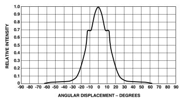
Figure 7. Relative luminous intensity vs. angular displacement for HLMP-Cx25 and HLMP-Cx27.
