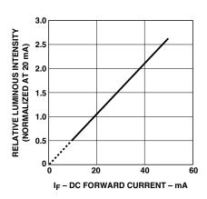
Figure 4. Relative luminous intensity vs. forward current.
