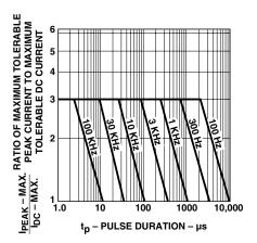
Figure 2. Maximum tolerable peak current vs. pulse duration.
