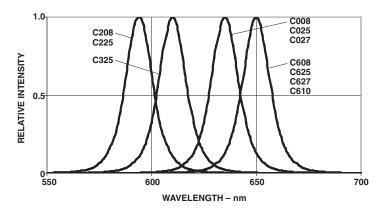
Figure 1. Relative intensity vs. wavelength.
