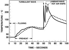
Figure 8. Recommended wave soldering profile.
