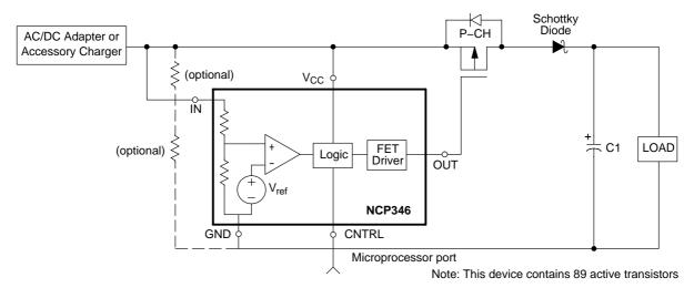
Figure 1. Simplified Application Diagram
