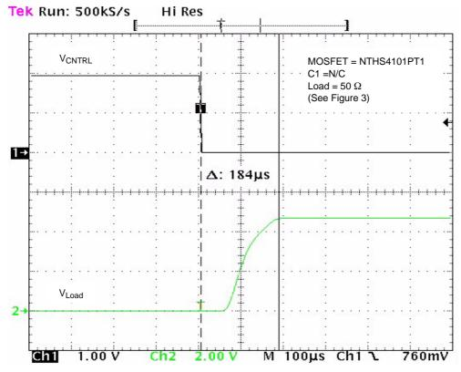
Figure 16. Typical Turn-on Time CNTRL (NCP346SN2)
