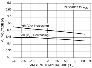
Figure 6. Typical Vth Variation vs. Temperature (NCP346SN2)
