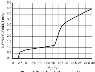
Figure 9. Total Supply Current vs. V<sub>CC</sub> (NCP346SN1)
