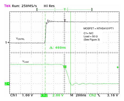
Figure 13. Typical Turn-off Time CNTRL (NCP346SN1)
