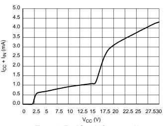
Figure 10. Total Supply Current vs. V<sub>CC</sub> (NCP346SN2)
