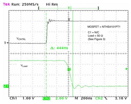
Figure 14. Typical Turn-off Time CNTRL (NCP346SN2)
