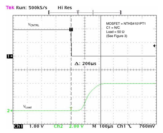
Figure 15. Typical Turn-on Time CNTRL (NCP346SN1)
