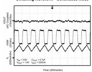
**Switching Waveform - Continuous Mode**
