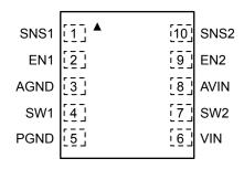
10-Pin 2mm x 2mm Thin MLF $^{\otimes}$  (MT) Fixed Output (Top View)
