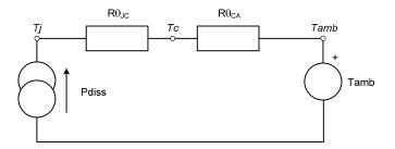
Now replacing the variables in the equation for Vx, we can find the junction temperature ( $T_J$ ) from power dissipation, ambient temperature and the known thermal resistance of the PCB ( $R\theta_{CA}$ ) and the package ( $R\theta_{JC}$ ):
