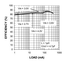
The figure above shows an efficiency curve. From no load to 100mA, efficiency losses are dominated by quiescent current losses, gate drive and transition losses. By using the HyperLight Load™ mode the MIC23254 is able to maintain high efficiency at low output currents.
