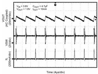
**Switching Waveform - Discontinuous Mode**
