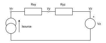
From this simple circuit we can calculate Vx if we know Isource, Vz and the resistor values, Rxy and Ryz using the equation:
