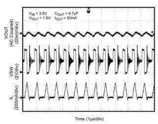
**Switching Waveform - Continuous Mode**
