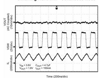
**Switching Waveform - Continuous Mode**
