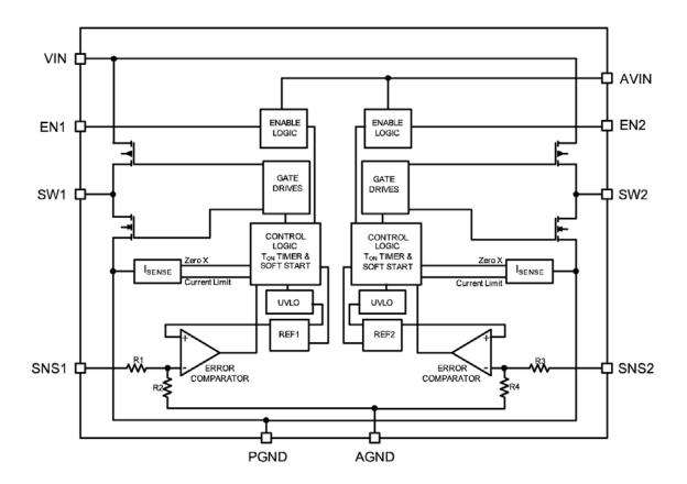
MIC23254 Simplified Fixed Output Block Diagram
