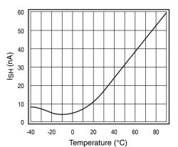
Figure 10. Shutdown Current vs. Temperature
