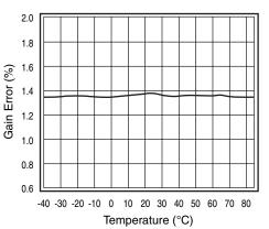
Figure 4. Gain Error vs. Temperature
