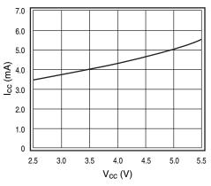
Figure 7. I<sub>CC</sub> vs. Supply Voltage
