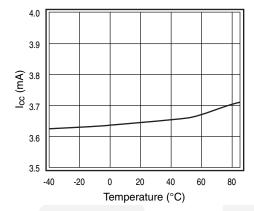
Figure 9. Supply Current vs. Temperature
