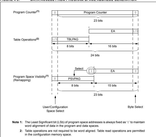
FIGURE 4-9: DATA ACCESS FROM PROGRAM SPACE ADDRESS GENERATION
