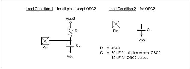
TABLE 30-15: CAPACITIVE LOADING REQUIREMENTS ON OUTPUT PINS
