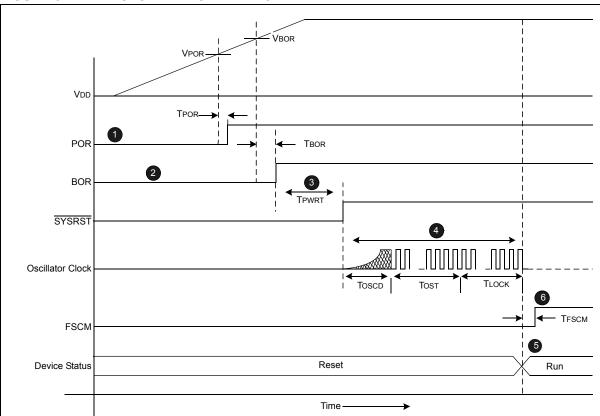
FIGURE 6-2: SYSTEM RESET TIMING
