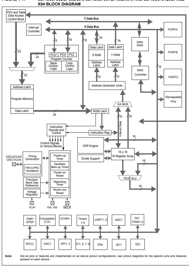
FIGURE 1-1: dsPIC33FJ32GP302/304, dsPIC33FJ64GPX02/X04, AND dsPIC33FJ128GPX02/
