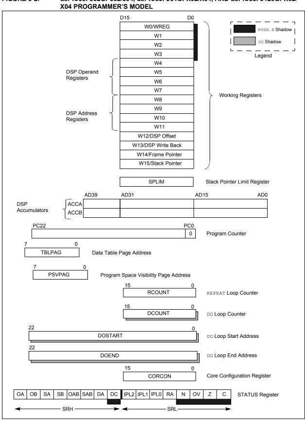
FIGURE 3-2: dsPIC33FJ32GP302/304, dsPIC33FJ64GPX02/X04, AND dsPIC33FJ128GPX02/
