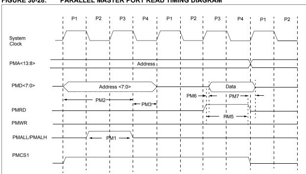
FIGURE 30-28: PARALLEL MASTER PORT READ TIMING DIAGRAM
