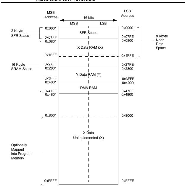
FIGURE 4-5: DATA MEMORY MAP FOR dsPIC33FJ128GP802/804 AND dsPIC33FJ64GP802/804 DEVICES WITH 16 KB RAM
