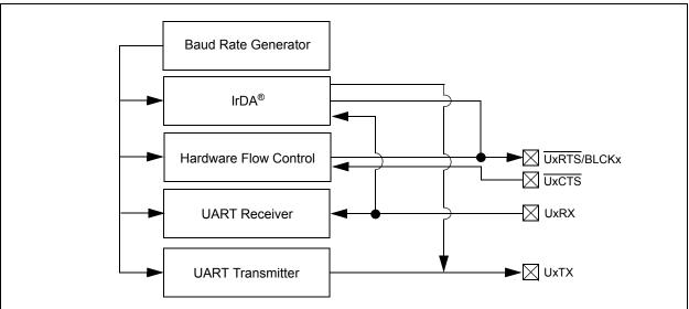
Note 1: Both UART1 and UART2 can trigger a DMA data transfer.
