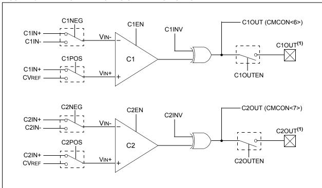
Note 1: This peripheral's outputs must be assigned to an available RPn pin before use. Refer to Section 11.6 "Peripheral Pin Select" for more information.
