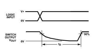
FIGURE 3A. MEASUREMENT POINTS
