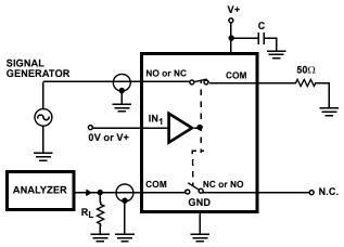
FIGURE 6. CROSSTALK TEST CIRCUIT
