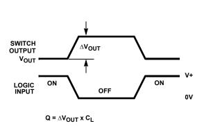
FIGURE 2A. MEASUREMENT POINTS
