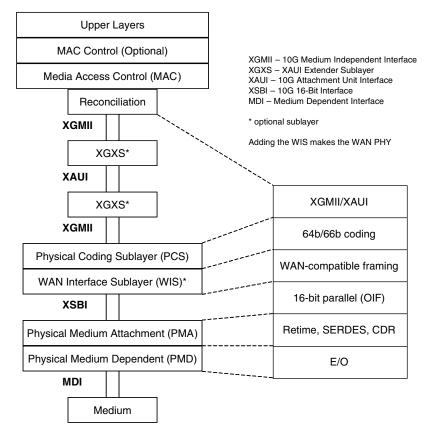
Figure 2-2. XAUI Solution Simplified Block Diagram
