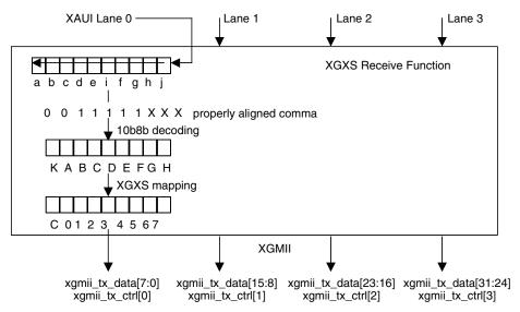
The transmit path, shown in Figure 2-6, is the data path from XGMII to XAUI. In the transmit direction, the 36-bit DDR data and control received at the XGMII are converted to single-edge timing and passed through an optional slip buffer that compensates for XAUI and XGMII timing differences. The XGMII data and control are then passed to the TX encoder, where they are translated and mapped to the 8b10b XAUI transmission code and then passed to the SERDES interface.
