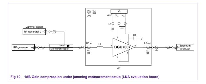
The gain was measured between port RFin and RFout of the EVB at the GPS frequency, while simultaneously a jammer power signal was swept at 20dB attenuated input of the directional coupler. Please note that the drive power of the jammer is 20dB lower at the input of the DUT caused by the directional coupler. Fig 11 and Fig 12 show the gain compression curves with 850MHz and 1850MHz jammers respectively.
