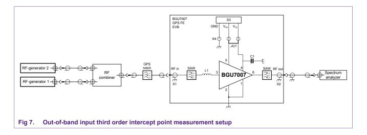
The input power levels of  $f_1$  and  $f_2$  that have been used to measure the IM3 levels on the front-end evaluation board were +10 dBm, shown in Fig 8. Fig 9 shows the IM3 level at the output of the front-end, measured at  $V_{CC}$  = 1.8 V.
