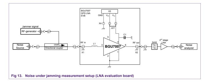
With the results of these measurements and the specification of the SAW filter, the jammer power levels that cause noise increase can be calculated.
