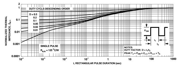
Figure 13. Transient Thermal Response Curve
