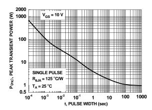
Figure 12. Single Pulse Maximum Power Dissipation
