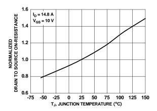
Figure 3. Normalized On-Resistance vs. Junction Temperature
