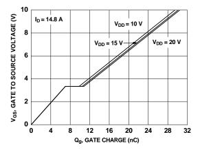
Figure 7. Gate Charge Characteristics
