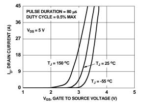
Figure 5. Transfer Characteristics
