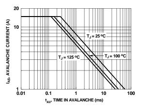
Figure 9. Unclamped Inductive Switching Capability
