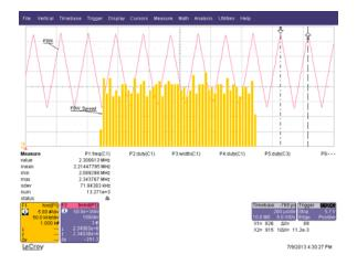
The modulation depth and modulation frequency are set by 2 external resistors to GND. The modulation frequency can be set from 5 kHz up to 50 kHz using a resistor from the RMOD pin to GND. The modulation depth can be set from 3% up to 30% of the nominal switching frequency using a resistor from the RDEPTH pin to GND. Please see the curves below for typical values:
