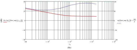
Figure 35. Bode Plot of the OTA Compensator
