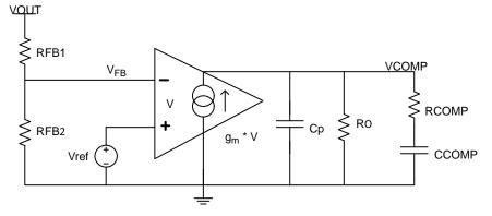
Figure 32. Feedback Compensator Network Model
