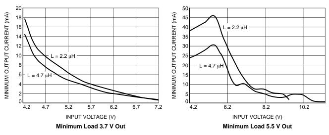
Figure 30. Minimum Load Current with Different Input and Output Voltages
