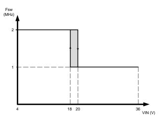
Figure 25. NCV890104 Switching Frequency Reduction at High Input Voltage
