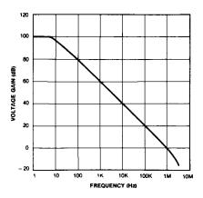
Figure 2. Open-Loop Frequency Response
