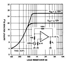
Figure 4. Output Voltage Swing vs Load Resistance
