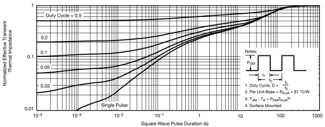
Normalized Thermal Transient Impedance, Junction-to-Ambient
