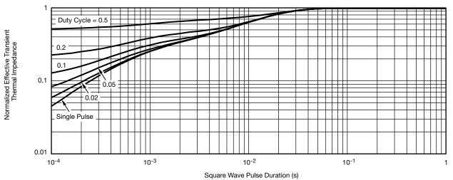
Normalized Thermal Transient Impedance, Junction-to-Case
