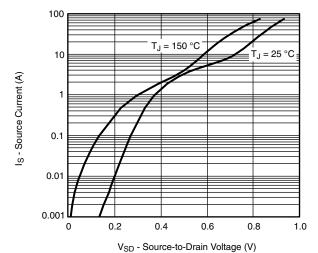
Source-Drain Diode Forward Voltage
