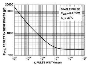
Figure 12. Single Pulse Maximum Power Dissipation
