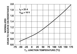
Figure 3. Normalized On-Resistance vs Junction Temperature
