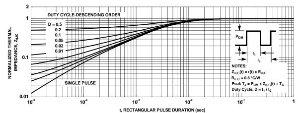
Figure 13. Junction-to-Case Transient Thermal Response Curve
