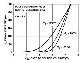
Figure 5. Transfer Characteristics
