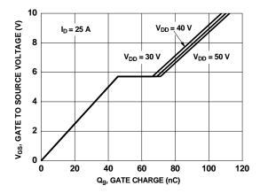
Figure 7. Gate Charge Characteristics
