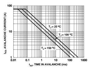
Figure 9. Unclamped Inductive Switching Capability
