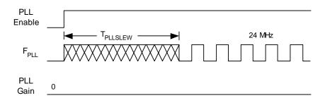
Figure 3-2. PLL Lock Timing Diagram
