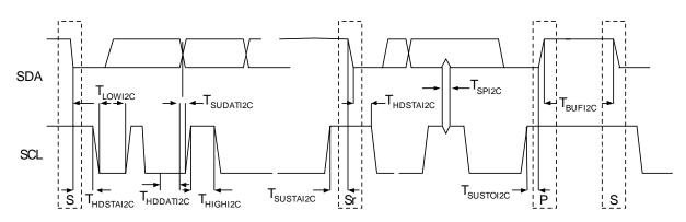
Figure 3-10. Definition for Timing for Fast/Standard Mode on the I<sup>2</sup>C Bus
