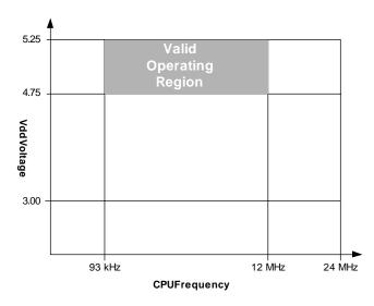
Figure 3-1. Voltage versus CPU Frequency
