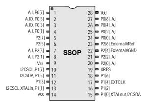
**LEGEND**: A = Analog, I = Input, and O = Output. \* These are the ISSP pins, which are not High Z at POR (Power On Reset). See the *PSoC Mixed-Signal Array Technical Reference Manual* for details.
