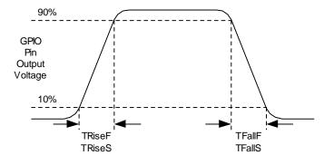
Figure 3-7. GPIO Timing Diagram
