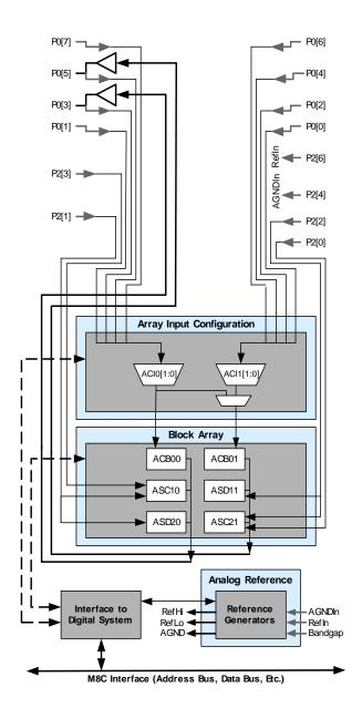
Analog System Block Diagram
