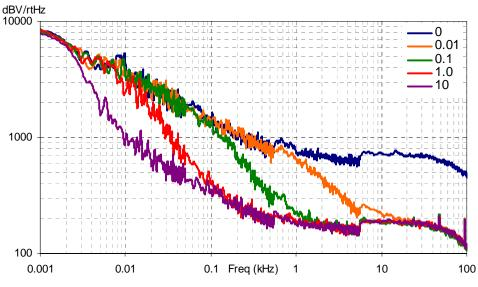
Figure 3-8. Typical AGND Noise with P2[4] Bypass
