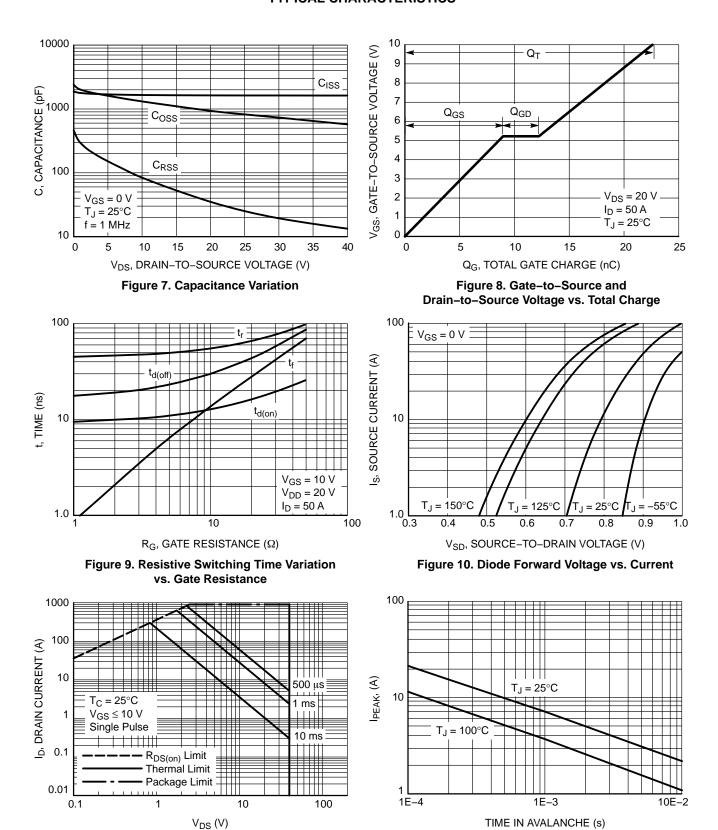
Figure 12. I<sub>PEAK</sub> vs. Time in Avalanche
