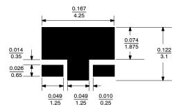
FIGURE 1. Recommended Copper Spreading Footprint
