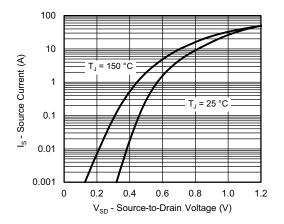
Source-Drain Diode Forward Voltage
