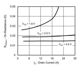
On-Resistance vs. Drain Current and Gate Voltage
