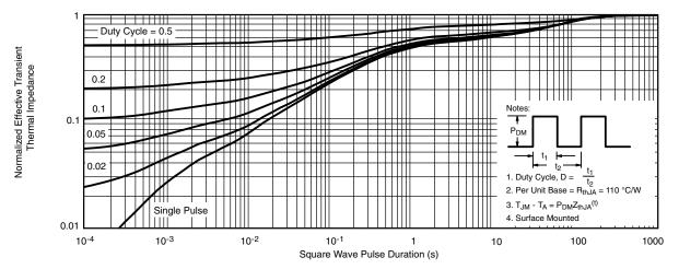
Normalized Thermal Transient Impedance, Junction-to-Ambient
