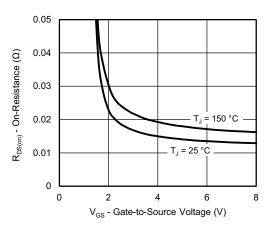
On-Resistance vs. Gate-to-Source Voltage
