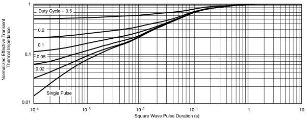
Normalized Thermal Transient Impedance, Junction-to-Case
