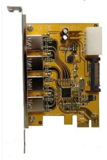
Renesas' third-generation Universal Serial Bus 3.0 host controller demonstration card, part number YET-D720201-0014, complies with the Universal Serial Bus 3.0 Specification (USB 3.0) and Intel's eXtensible Host Controller Interface (xHCI). The demonstration card supports up to four Super-Speed USB 3.0 ports. This demonstration card uses a PCI Express® Gen 2 system interface bus, which makes it easy to add multiple SuperSpeed ports to systems containing a PCI Express bus interface.
