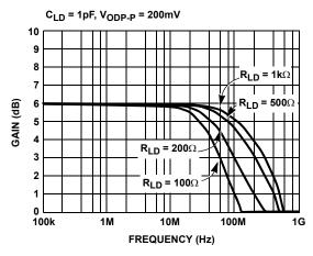
FIGURE 2. SMALL SIGNAL FREQUENCY RESPONSE vs  $R_{LD}$
