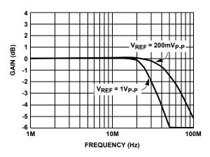
FIGURE 4. FREQUENCY RESPONSE vs V<sub>REF</sub>
