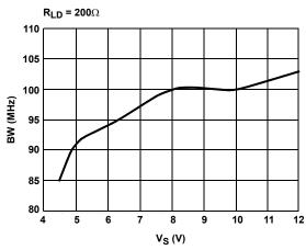
FIGURE 10. BANDWIDTH vs SUPPLY VOLTAGE
