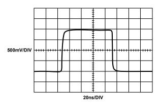
FIGURE 14. LARGE SIGNAL TRANSIENT RESPONSE
