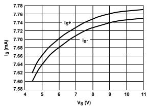
FIGURE 11. SUPPLY CURRENT vs SUPPLY VOLTAGE
