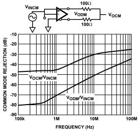
FIGURE 6. COMMON MODE REJECTION vs FREQUENCY
