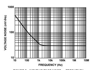
FIGURE 8. INPUT VOLTAGE NOISE vs FREQUENCY
