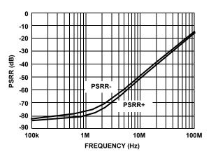
FIGURE 5. POWER SUPPLY REJECTION RATIO vs FREQUENCY
