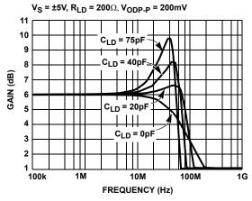
FIGURE 3. SMALL SIGNAL FREQUENCY RESPONSE vs CLD
