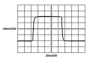
FIGURE 15. SMALL SIGNAL TRANSIENT RESPONSE
