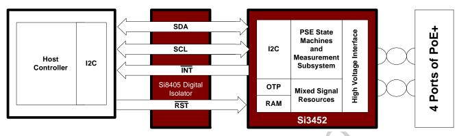
Figure 2. 4-Port System with Direct Host Connection
