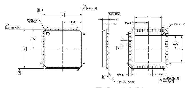
Figure 7. 40-Pin QFN Mechanical Diagram
