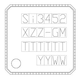
Figure 9. Device Marking Diagram
