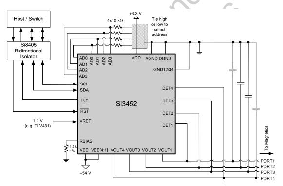
Figure 3. 4-Port Application Diagram Using dV/dt Disconnect and I<sup>2</sup>C Host Interface
