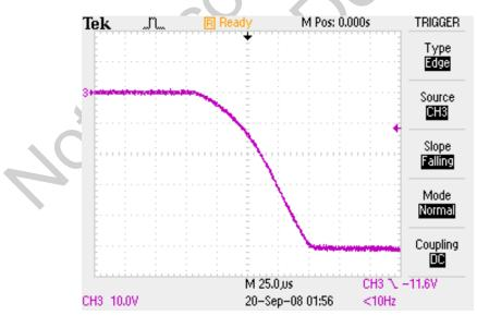
Figure 5. Turn-On Waveform—Vport Relative to GND
