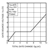
Fig.3 Dynamic Input Characteristics
