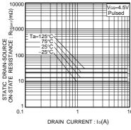
Fig.8 Static Drain-Source On-State Resistance vs. Drain Current (2)
