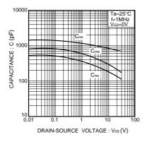
Fig.1 Typical Capacitance vs. Drain-Source Voltage
