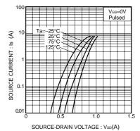
Fig.6 Source-Current vs. Source-Drain Voltage
