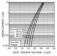
Fig.4 Typical Transfer Characteristics
