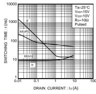
Fig.2 Switching Characteristics
