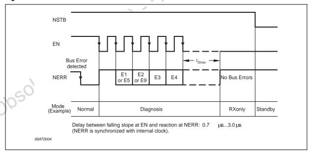
Readout is initialized by a negative edge on EN and acknowledged by NERR entering HIGH state. Following the next negative edge the first error status bit is displayed on NERR according to the data table below. If no
