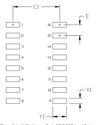
Figure 7.1. 16-Pin Narrow Body SOIC PCB Land Pattern
