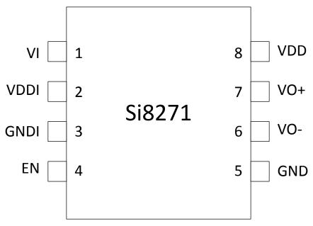
Figure 5.1. Pin Assignments Si8271
