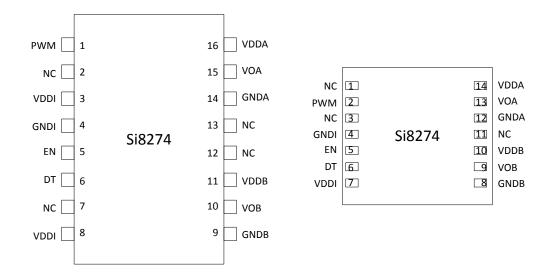
Figure 5.3. Pin Assignments Si8274
