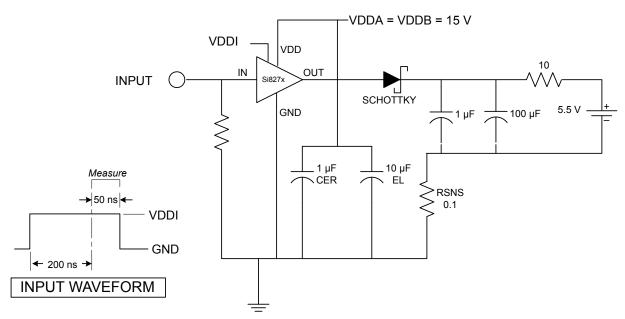
Figure 4.2. IOH Source Current Test Circuit
