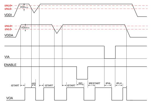
Figure 2.18. Device Behavior during Normal Operation and Shutdown
