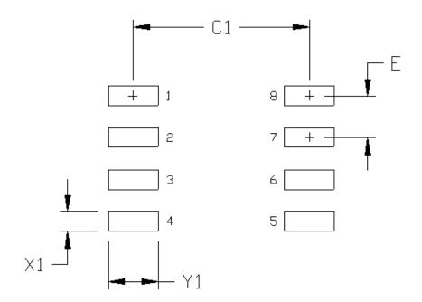
Figure 7.2. 8-Pin Narrow Body SOIC Land Pattern
