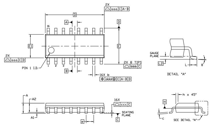
Figure 6.1. 16-pin Small Outline Integrated Circuit (SOIC) Package
