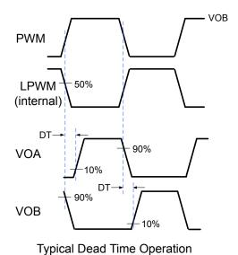
Figure 2.20. Dead Time Waveforms for Si8274 Drivers
