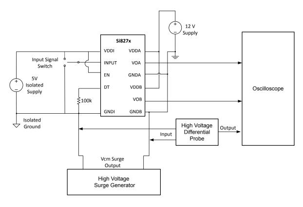
Figure 4.3. Common Mode Transient Immunity Test Circuit
