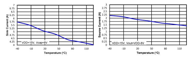
Figure 2.15. Output Sink Current vs. Temperature
