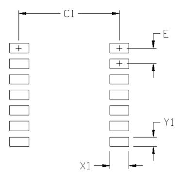
Figure 7.3. 14-Pin QFN Land Pattern
