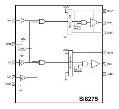
Figure 2.4. Si8275 Block Diagram
