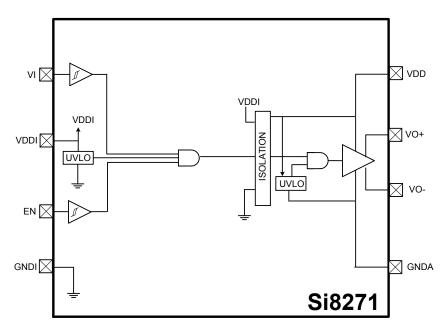
Figure 2.1. Si8271 Block Diagram
