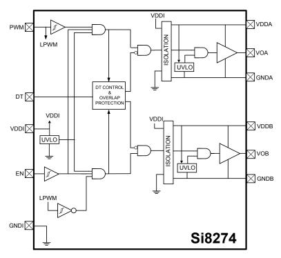
Figure 2.3. Si8274 Block Diagram
