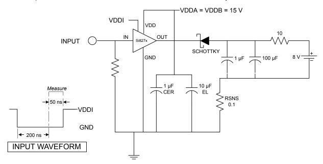
Figure 4.1. IOL Sink Current Test Circuit
