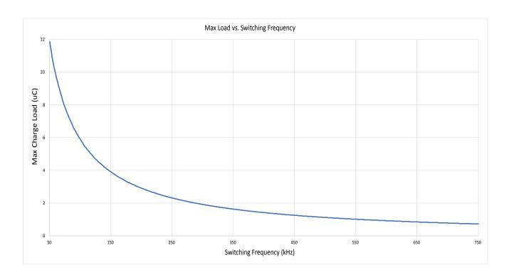
Figure 2.17. Max Load vs. Switching Frequency
