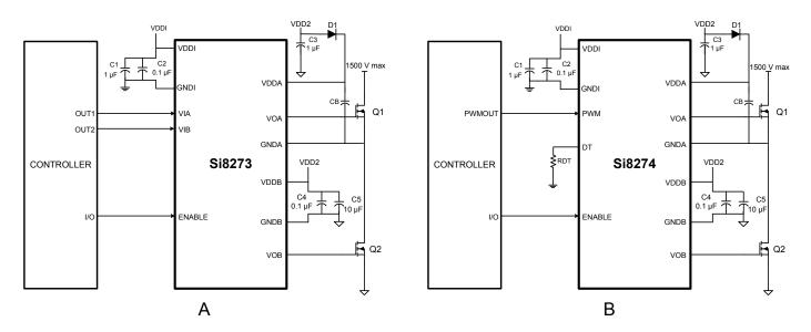
Figure 3.1. Si827x in Half-Bridge Application
