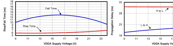
Figure 2.7. Rise/Fall Time vs. Supply Voltage
