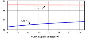
Figure 2.8. Propagation Delay vs. Supply Voltage
