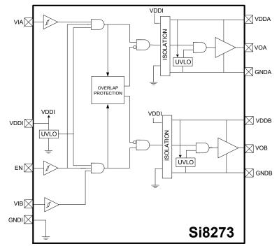
Figure 2.2. Si8273 Block Diagram
