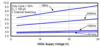
Figure 2.9. Supply Current vs. Supply Voltage
