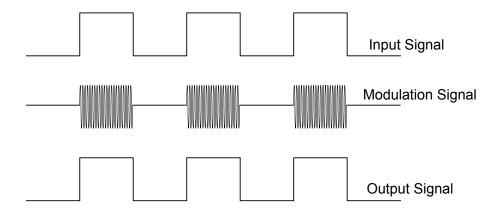
Figure 2.6. Modulation Scheme
