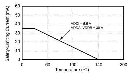
Figure 4.5. NB SOIC-8 Thermal Derating Curve, Dependence of Safety Limiting Values
