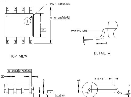
Figure 6.2. 8-Pin Narrow Body SOIC Package
