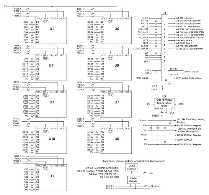
Note: 1. The ZQ ball on each DDR4 component is connected to an external  $240\Omega \pm 1\%$  resistor that is tied to ground. It is used for the calibration of the component's ODT and output driver.
