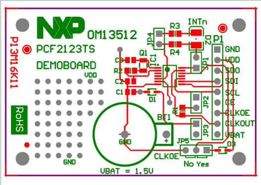
Fig 4. Demo board and top side layout
