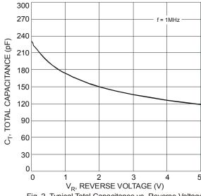
Fig. 2 Typical Total Capacitance vs. Reverse Voltage
