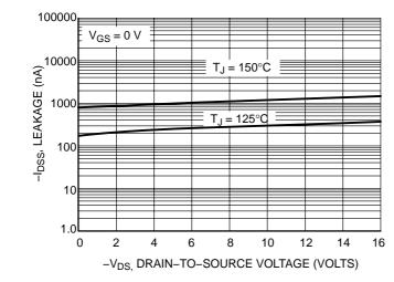
Figure 10. Drain-to-Source Leakage Current vs. Voltage
