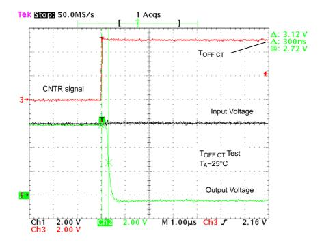
Figure 17. T<sub>OFF CT</sub> Waveforms
