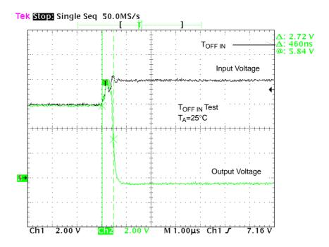
Figure 14.  $T_{OFF\ IN}$  Waveforms
