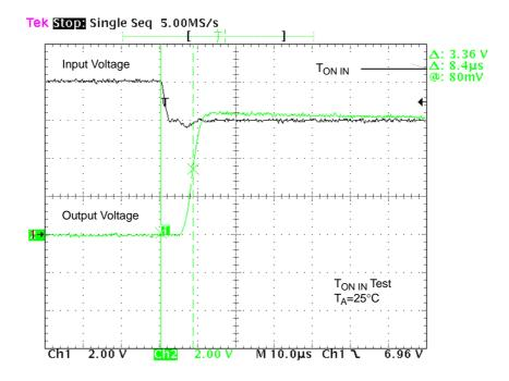
Figure 13. T<sub>ON IN</sub> Waveforms
