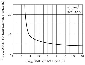
Figure 5. On–Resistance vs. Gate–to–Source Voltage
