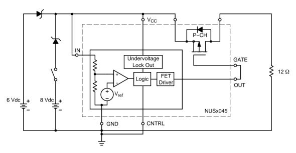
Figure 12. Test Circuit for Ton In and Toff In
