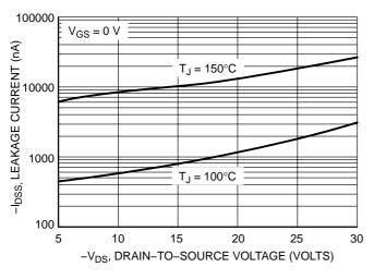
Figure 6. Drain-to-Source Leakage Current vs. Voltage
