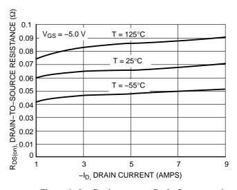
Figure 9. On–Resistance vs. Drain Current and Temperature
