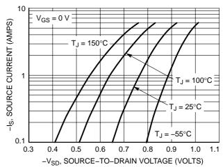
Figure 7. Diode Forward Voltage vs. Current
