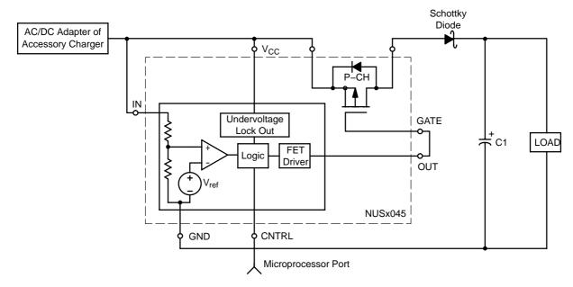
Figure 1. Simplified Schematic
