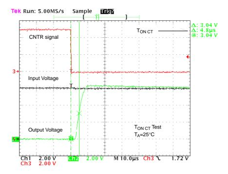
Figure 16. T<sub>ON CT</sub> Waveforms
