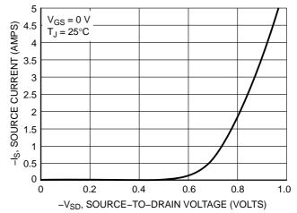
Figure 11. Diode Forward Voltage vs. Current
