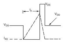
Fig. 12b - Unclamped Inductive Waveforms
