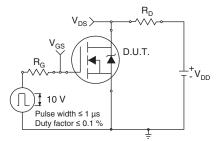
Fig. 10a - Switching Time Test Circuit
