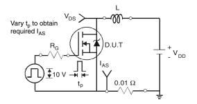
Fig. 12a - Unclamped Inductive Test Circuit
