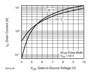
Fig. 3 - Typical Transfer Characteristics
