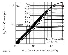
Fig. 2 - Typical Output Characteristics, T<sub>C</sub> = 175 °C
