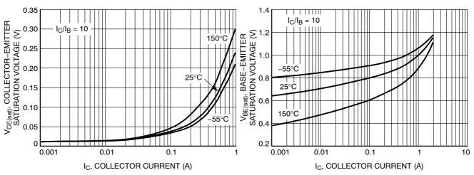
Figure 3. Collector Emitter Saturation Voltage vs. Collector Current
