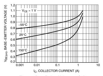
Figure 5. Base Emitter Voltage vs. Collector
