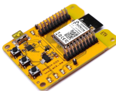
AMW004-E03 ‘Mackerel’ (with AMW004 surface mount module)
