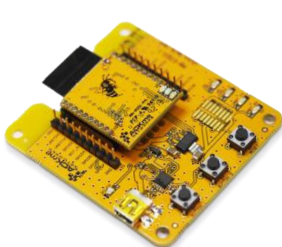
AMW004-E02 ‘Marlin’ (with AMW004-A01 through-hole module adapter)
