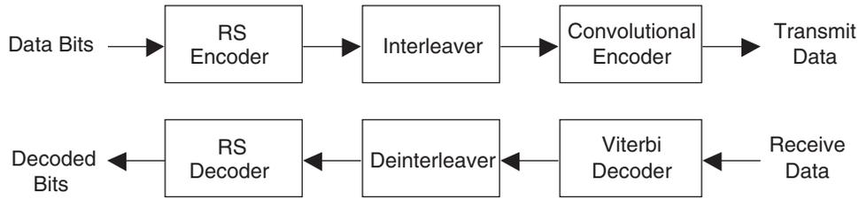
A Reed-Solomon Decoder can correct errors and erasures. The maximum number of correctable erroneous symbols in a codeword is  $t = (n-k)/2$ , and the maximum number of correctable erasures in a codeword is  $\mu = n-k$ .
