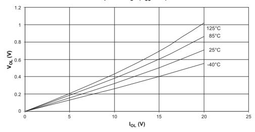
Figure 22-21. I/O Pin Source Current versus Output Voltage ( $V_{CC} = 5V$ )
