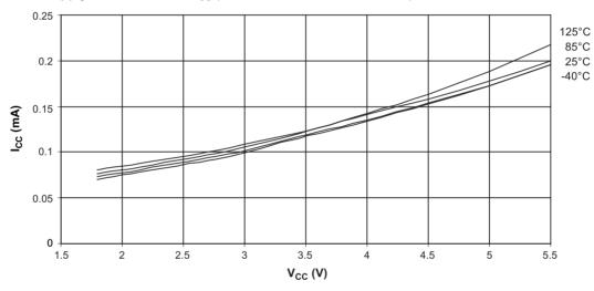
Figure 22-9. Idle Supply Current versus  $V_{CC}$  (Internal RC Oscillator, 1MHz)
