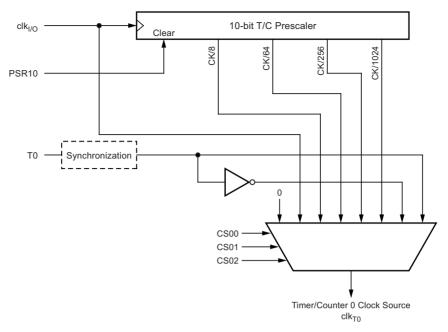
Note: 1. The synchronization logic on the input pins (T0) is shown in Figure 12-1.
