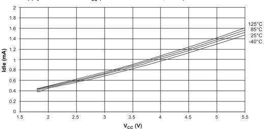
Figure 22-10. Idle Supply Current versus V<sub>CC</sub> (Internal RC Oscillator, 8MHz)
