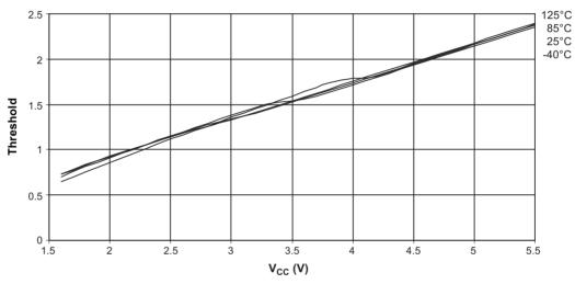
Figure 22-29. Reset Input Threshold Voltage versus V<sub>CC</sub> (VIL, Reset Pin Read As '0')
