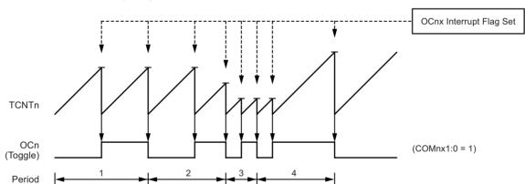
Figure 11-5. CTC Mode, Timing Diagram
