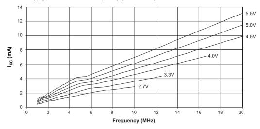
Figure 22-3. Active Supply Current versus V<sub>CC</sub> (Internal RC Oscillator, 128kHz)
