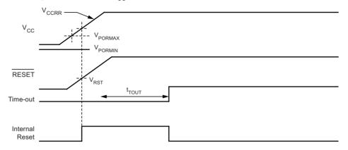
Figure 7-3. MCU Start-up, RESET Extended Externally
