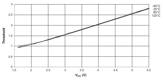
Figure 22-26. I/O Pin Input Threshold Voltage versus  $V_{CC}$  (VIL, I/O Pin Read As '0')
