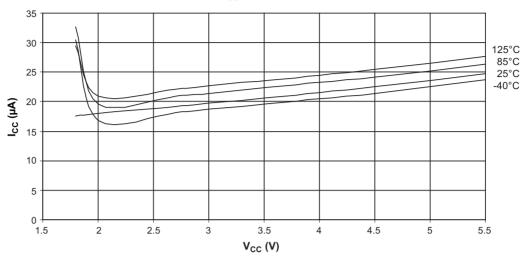
Figure 22-40. Analog Comparator Current versus V<sub>CC</sub>
