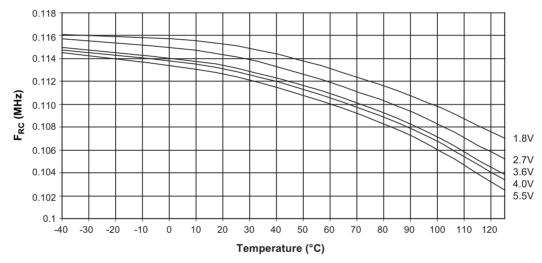
Figure 22-36. Calibrated 8MHz RC Oscillator Frequency versus Temperature
