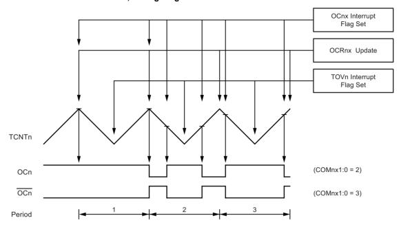
The Timer/Counter overflow flag (TOV0) is set each time the counter reaches BOTTOM. The interrupt flag can be used to generate an interrupt each time the counter reaches the BOTTOM value.
