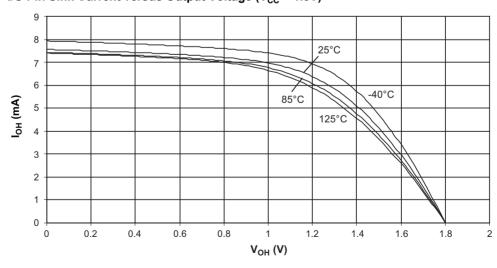
Figure 22-23. I/O Pin Sink Current versus Output Voltage ( $V_{CC} = 3V$ )
