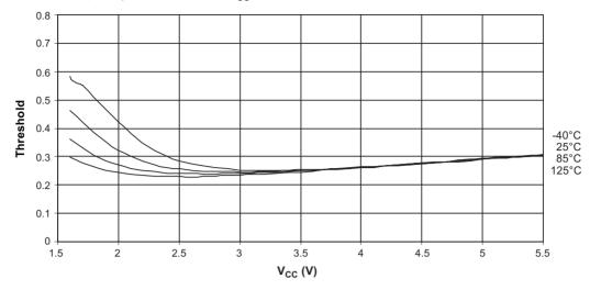
Figure 22-28. Reset Input Threshold Voltage versus V<sub>CC</sub> (VIH, Reset Pin Read As '1')
