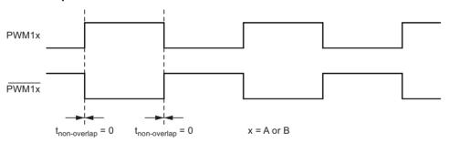
When the counter value match the contents of OCR1A or OCR1B, the OC1A and OC1B outputs are set or cleared according to the COM1A1/COM1A0 or COM1B1/COM1B0 bits in the Timer/Counter1 control register A - TCCR1, as shown in Table 13-4 on page 83.
