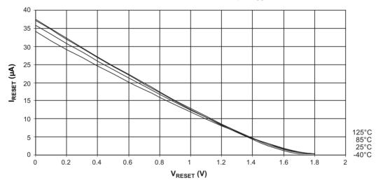
Figure 22-17. Reset Pull-Up Resistor Current versus Reset Pin Voltage ( $V_{CC} = 2.7V$ )
