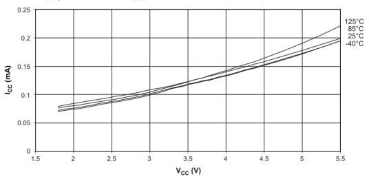
Figure 22-4. Active Supply Current versus V<sub>CC</sub> (Internal RC Oscillator, 1MHz)
