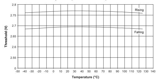
Figure 22-33. BOD Thresholds versus Temperature (BODLEVEL Is 1.8V)
