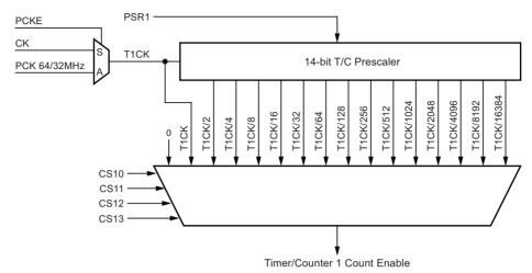
In the asynchronous clocking mode the clock selections are from PCK to PCK/16384 and stop, and in the synchronous clocking mode the clock selections are from CK to CK/16384 and stop. The clock options are described in Table 13-2 on page 78 and the Timer/Counter1 control register, TCCR1. Setting the PSR1 bit in GTCCR register resets the prescaler. The PCKE bit in the PLLCSR register enables the asynchronous mode. The frequency of the fast peripheral clock is 64MHz (or 32MHz in low speed mode).
