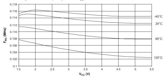
Figure 22-35. Watchdog Oscillator Frequency versus Temperature
