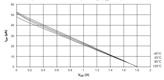
Figure 22-14. I/O Pin Pull-Up Resistor Current versus Input Voltage ( $V_{CC} = 2.7V$ )
