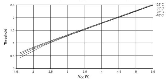
Figure 22-27. I/O Pin Input Hysteresis versus  $V_{CC}$
