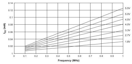
Figure 22-42. Reset Supply Current versus V<sub>CC</sub> (1 to 24MHz, Excluding Current through the Reset Pull-up)
