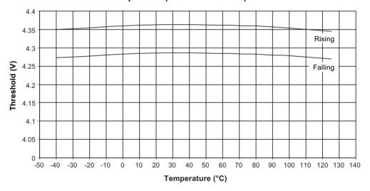
Figure 22-32. BOD Thresholds versus Temperature (BODLEVEL Is 2.7V)
