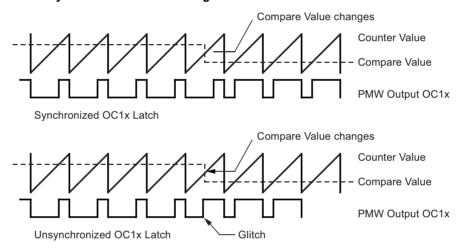
During the time between the write and the latch operation, a read from OCR1A or OCR1B will read the contents of the temporary location. This means that the most recently written value always will read out of OCR1A or OCR1B.
