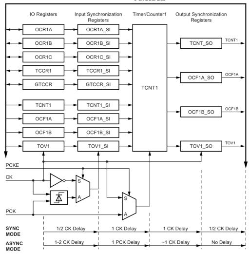
Timer/Counter1 and the prescaler allow running the CPU from any clock source while the prescaler is operating on the fast 64MHz (or 32MHz in low speed mode) PCK clock in the asynchronous mode.
