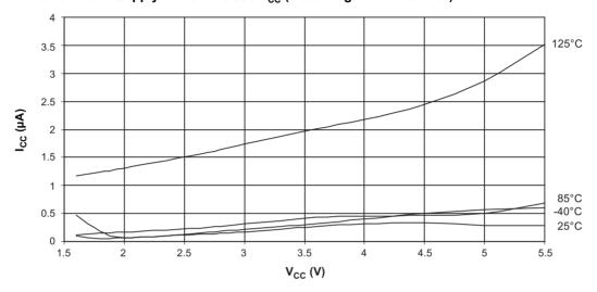
Figure 22-12. Power-Down Supply Current versus V<sub>CC</sub> (Watchdog Timer Enabled)
