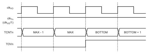
Figure 11-9 shows the same timing data, but with the prescaler enabled.
