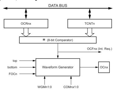
The OCR0x registers are double buffered when using any of the pulse width modulation (PWM) modes. For the normal and clear timer on compare (CTC) modes of operation, the double buffering is disabled. The double buffering synchronizes the update of the OCR0x compare registers to either top or bottom of the counting sequence. The synchronization prevents the occurrence of odd-length, non-symmetrical PWM pulses, thereby making the output glitch-free.
