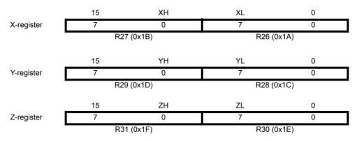
In the different addressing modes these address registers have functions as fixed displacement, automatic increment, and automatic decrement (see the instruction set reference for details).
