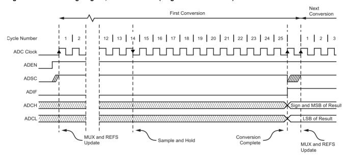
Figure 17-5. ADC Timing Diagram, Single Conversion
