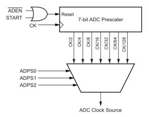
By default, the successive approximation circuitry requires an input clock frequency between 50kHz and 200kHz to get maximum resolution. If a lower resolution than 10 bits is needed, the input clock frequency to the ADC can be higher than 200kHz to get a higher sample rate. It is not recommended to use a higher input clock frequency than 1MHz.
