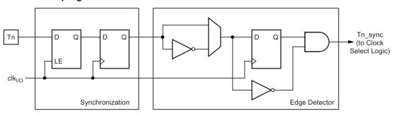
The synchronization and edge detector logic introduces a delay of 2.5 to 3.5 system clock cycles from an edge has been applied to the T0 pin to the counter is updated.
