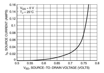
Figure 9. Diode Forward Voltage vs. Current
