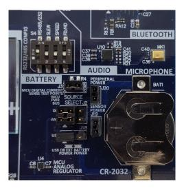
NOTE: For the purposes of this Out-of-Box Demo, ensure the jumper at J17 (BOOT MODE) is not installed across the pins.
