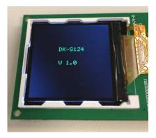
After 2 seconds, the screen will change to the measurement screen shown below. The SSP Out-Of-Box Demo application uses the A/D converter to read the voltage values present on the Potentiometer (POT1), the Light Sensor U8 (APDS-9005) and the Temperature Sensor U9 (TMP35). The program displays the raw hex value read from the Light Sensor and the Potentiometer. It converts the raw value read from the Temperature Sensor to the equivalent Fahrenheit temperature.
