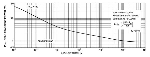
Figure 11. Single Pulse Maximum Power Dissipation
