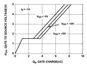
Figure 7. Gate Charge Characteristics
