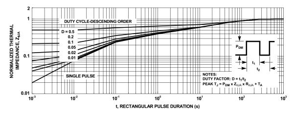
Figure 12. Transient Thermal Response Curve
