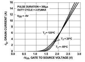
Figure 5. Transfer Characteristics
