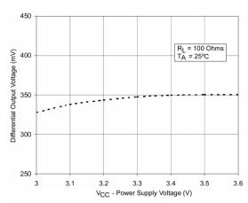
Figure 8. Differential Output Voltage vs. Power Supply Voltage
