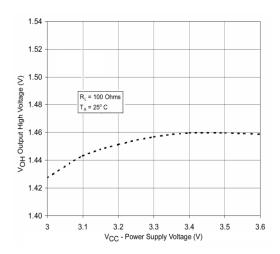
Figure 5. Output High Voltage vs. Power Supply Voltage
