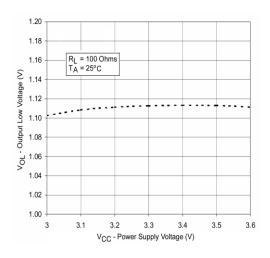
Figure 6. Output Low Voltage vs. Power Supply Voltage
