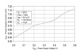
Figure 12. Power Supply Current vs. Power Supply Voltage
