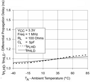
Figure 15. Differential Propagation Delay vs. Ambient Temperature
