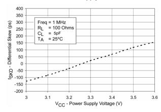
Figure 16. Differential Pulse Skew (tplh - tphl) vs. Power Supply Voltage
