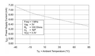
Figure 13. Power Supply Current vs. Ambient Temperature
