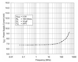
Figure 11. Power Supply Current vs. Frequency
