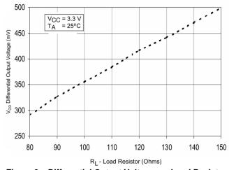
Figure 9. Differential Output Voltage vs. Load Resistor
