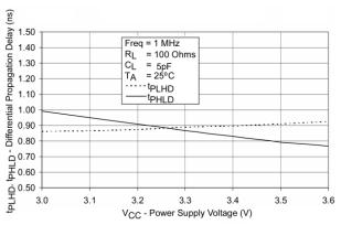
Figure 14. Differential Propagation Delay vs. Power Supply
