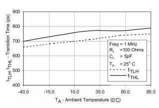
Figure 19. Transition Time vs. Ambient Temperature
