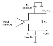
Note A: All input pulses have frequency = 10 MHz,  $t_R$  or  $t_F$  = 2 ns Note B:  $C_L$  includes all probe and fixture capacitances
