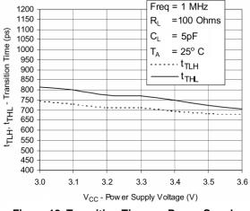
Figure 18. Transition Time vs. Power Supply Voltage
