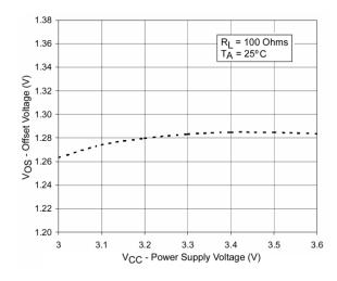
Figure 10. Offset Voltage vs. Power Supply Voltage
