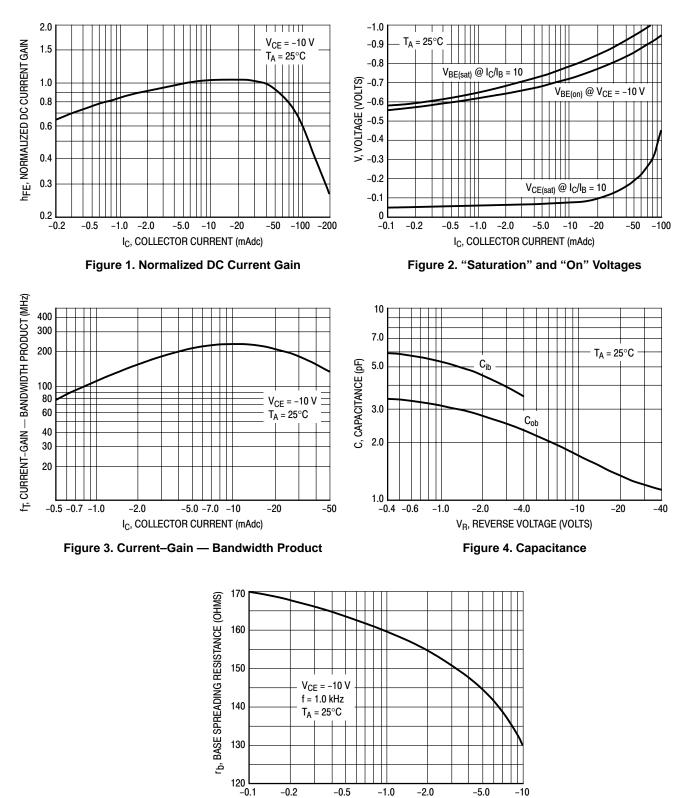
I<sub>C</sub>, COLLECTOR CURRENT (mAdc) Figure 5. Base Spreading Resistance
